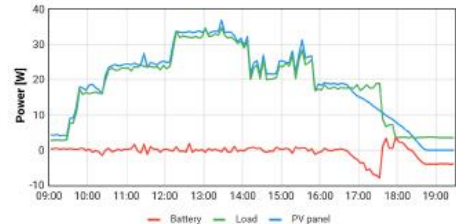
Figure 5.4: Charging process of several cubes over one day, data averaged over a 5 minutes interval
